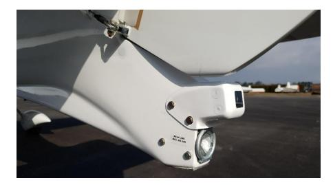
The max. permissible towing load is up to 850 kg! The banner size can be up to 200m <sup>2</sup> surface area with a max. 20 kg weight allowed. Optionally, for the DYNAMIC WT 9, currently the only tow plane of this class, an electrical cable retraction device (TOST system) is available.
