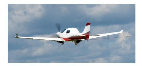
**Aircraft towing + banner towing-** The low weight and perfect aerodynamics result in towing capacities, which are equal or superior to conventional GA tow aircraft that are driven by 180 HP engines. The benefits are obvious as there is a 50% reduction in fuel costs and a significantly lower purchase price when compared to larger GA aircraft.
