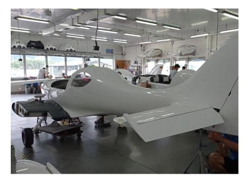
The cruising speed of the DYNAMIC WT9 depends on the respective engine and equipment (power at approx. 75%) the speed ranges from approx. 120 ktas to approx. 167 ktas. The take-off roll is very short at 142m while a short field landing can achieve 123m.
